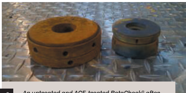
An untreated and ACE-treated RotaChock® after salt spray test
